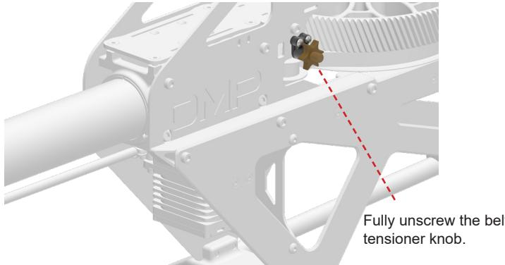
**!** Pay close attention when installing the belt. Ensure that both sides of the belt are running parallel. The belt must not be twisted in itself. Rotate the free end of the belt 90° as depicted by the arrow in the picture. Once you have achieved the state shown in the picture, insert the belt into the frame and loop it around the main belt pulley.
