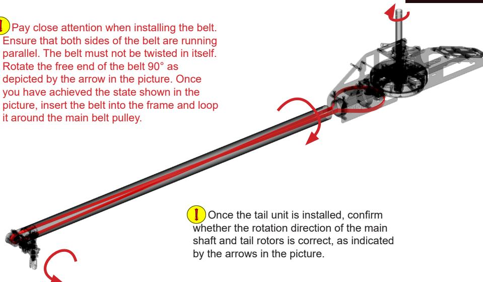
**!** Once the tail unit is installed, confirm whether the rotation direction of the main shaft and tail rotors is correct, as indicated by the arrows in the picture.
