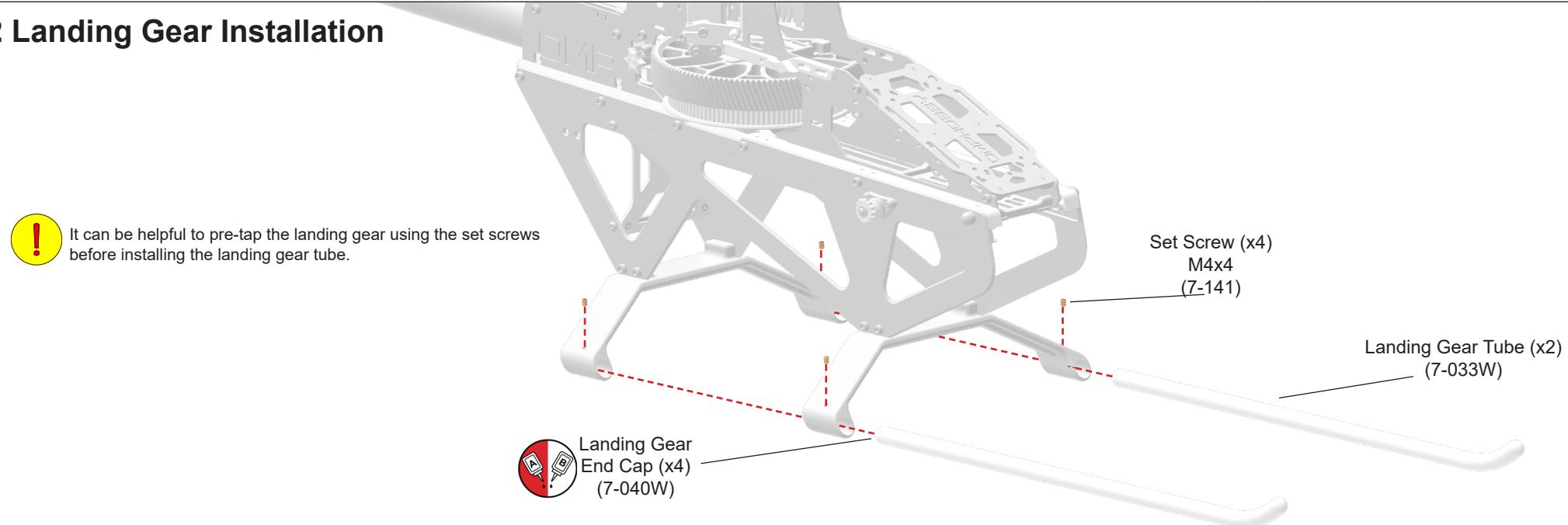
! It can be helpful to pre-tap the landing gear using the set screws before installing the landing gear tube.
