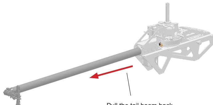
Pull the tail boom back until the belt has no slack remaining, but no further.
