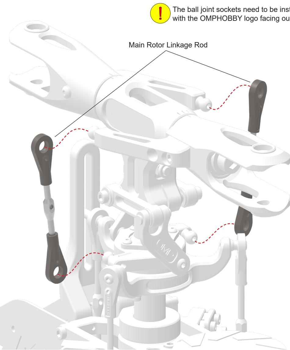
**!** The ball joints are intentionally manufactured tight to prevent slop, they can be freed up by gently squeezing them with flat-jaw pliers when installed on the ball. Never use serrated pliers.
