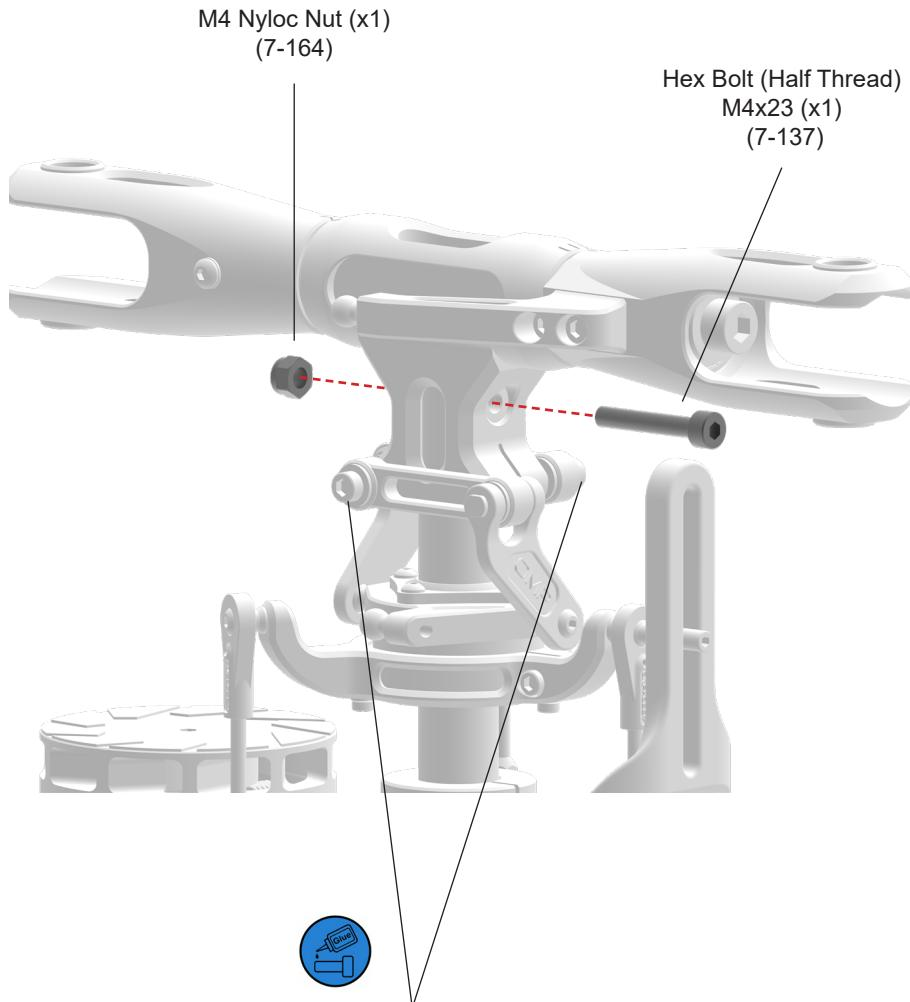
**!** The swashplate driver arm screws must be tightened in this step to clamp the main rotor yoke onto the main shaft. To ensure proper alignment, first install the M4x23 Hex Bolt, but don't fully tighten yet, and then tighten the swashplate driver arm screws with thread locker evenly and in small steps. After that, don't forget to fully tighten the M4x23 Hex Bolt.
