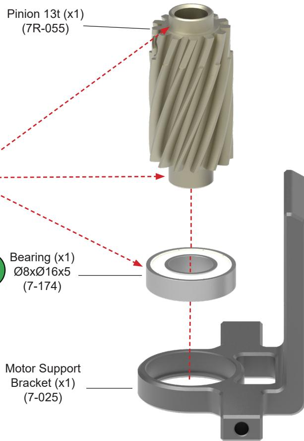
We recommend cleaning the marked pinion parts, inner and outer bearing races and bearing seat of the motor support bracket, and to apply a very small amount of High Strength LOCTITE® (e.g. 638) to prevent wear in these areas.
